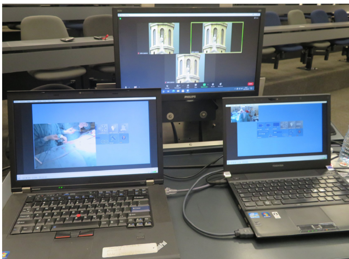
Figure 5: In the remote auditorium, we make use of two further laptops running a media player which can output to the data projector for the audience with the Zoom link shown in the top screen for audio communication
